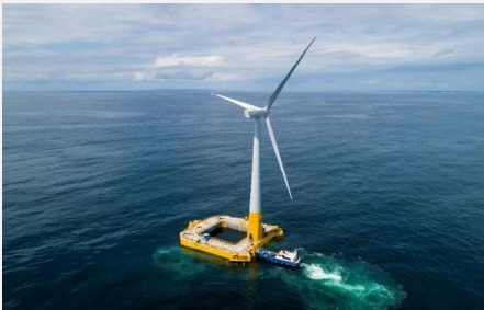
Figure 2 Example of a barge floating substructure. Image courtesy of BW Ideal. All rights reserved.
